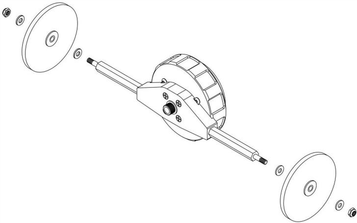
Remove outer wheels using 7/16" wrench
