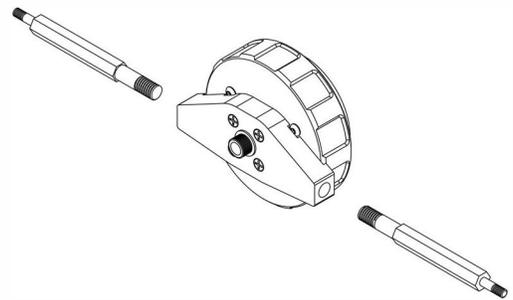
Remove axles using 1/2" wrench
